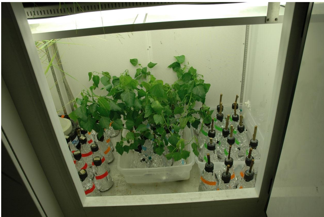
Figure B-9 Experimental set up for hydroponic exposure experiment with hybrid poplar in growth chamber.
