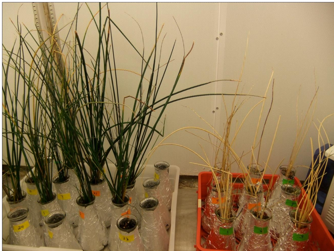
Figure A-7 Experimental set up for hydroponic exposure experiment with softstem bulrush in growth chamber.
